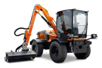
The T telescopic arm has been designed to work with an extension up to 6,7 meters and to reach a maximum height of 8,6 meters. Its particular geometry enhances the characteristics for road maintenance where you want a combination of mowing roadside and finishing work far from the roadside. The sturdy telescopic extension of the model T6.5 allows greater work agility and maximum performance even in difficult situations.
