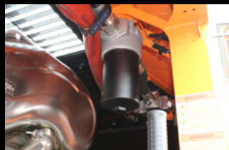
Drain filter for travel and mulcher circuit
