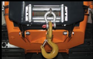
Rear winch with 6 t pulling power
