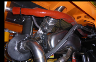
Second stage air filtration with ejector
