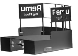
The REMU counterweight can be equipped with an inbuilt fuel tank to refuel the original.
