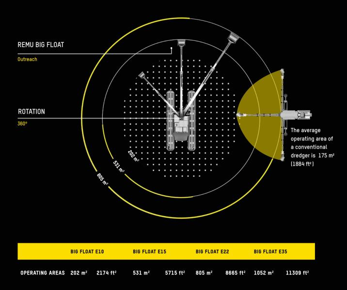
The operating area of the Big Float amphibious excavator is superior compared to traditional dredgers. Depending on the model and boom length, the outreach in front is according of boom system and base machine.
